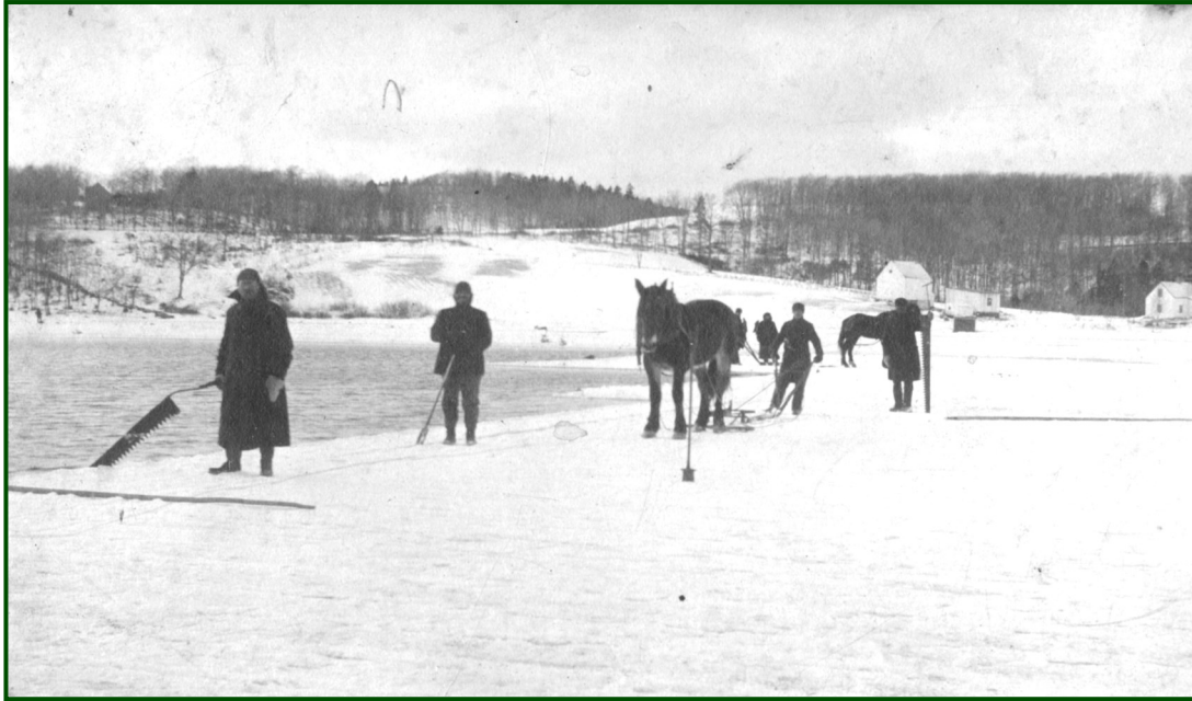
Cutting blocks of ice with the saw and then using horses to transport them. C.F. Bell Collection, DHM
